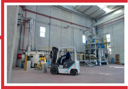
We prioritize energy efficiency while obtaining a total of 1300 kg of liquid aluminum per hour with our main melting furnaces with shaft type and promeos burner system in our melting department. The liquid metal melted in our furnaces is cleaned with an automatic degassing machine and made ready to produce porosity-free parts.
